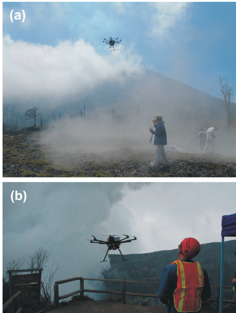
Figure 1. A DJI S1000 octocopter flying at Turrialba volcano in April 2017. (a) During takeoffs and landings, the loose volcanic ash on the ground is stirred into the air by the drone's rotors. This constitutes a potential hazard for the drone's motors and for the instrumentation. Note the white clouds and the blue-tinged volcanic gas in the background, with the 3,340-m summit of the volcano in the distance. (b) The S1000 landing at the summit mirador on 26 April 2017, with strong degassing from the summit craters evident in the background.
