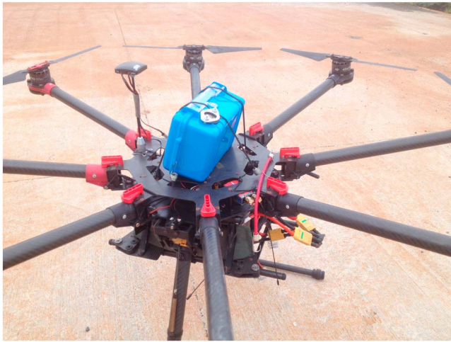
Figure 4. Photo showing the DROAS instrument mounted upon the S1000 octocopter. Note that the telescope of the DROAS is angled \sim 15^\circ from vertical, in order to compensate for the position of the drone when flying, which is tilted slightly forward relative to horizontal.
