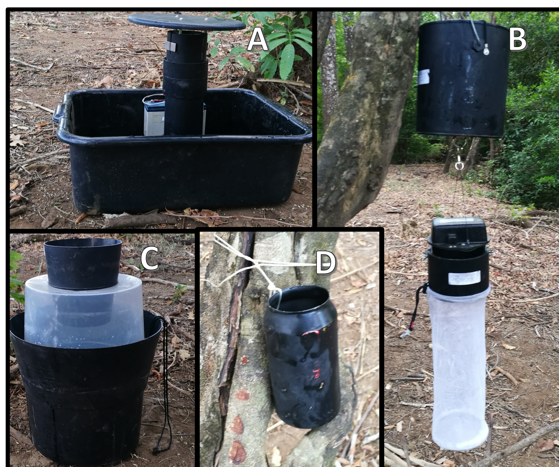
Figure 3. Vector traps. A: CDC Gravid Traps (GT) (Jonh W. Hock®). B: Encephalitis vector Surveillance Traps (EVS) (Bioquip®). C: Gravid Aedes Trap (BG-GAT) (Biogents®). D: Ovi-trap
