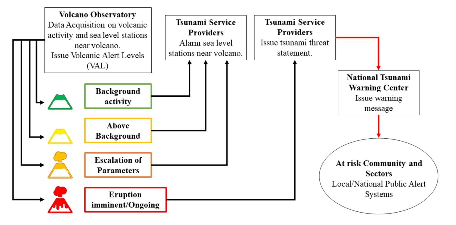
The Intergovernmental Coordination Group for the Tsunami and other Coastal Hazards Warning System for the Caribbean and Adjacent Regions (ICG/CARIBE-EWS) Task Team on Volcanic Sources proposed schematic for alerting on tsunamis generated by volcanoes based on the established VAL in addition to data from sea level stations.
