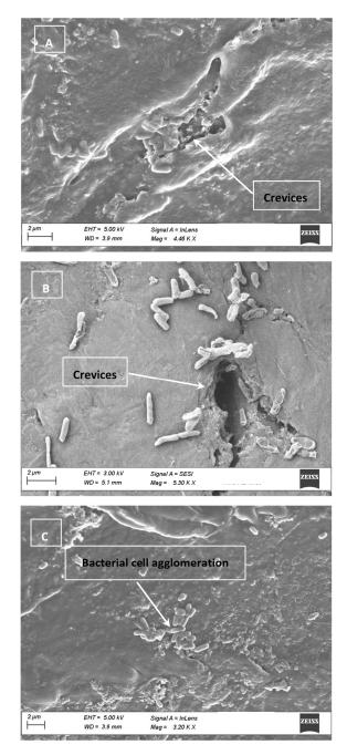
**Figure 3.** (**A**–**C**) Electron micrograph of three different high-density polyethylene (HD) samples used during the experiments. Based on the scale indicated in the micrograph, the crevice highlighted in (**B**) appears to be large enough to harbor *Salmonella* cells (rod shaped). (**C**) depicts bacterial cell agglomerates present on the surface of the HD.
