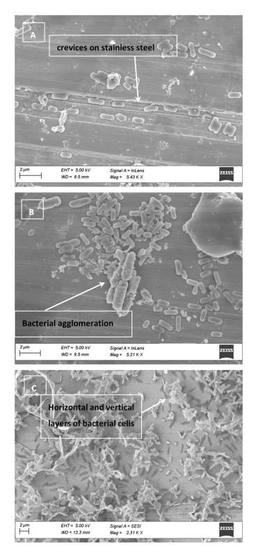
**Figure 2.** Electron micrograph of stainless steel (SS) inoculated with *Salmonella* showing imperfections on SS (**A**) and agglomeration of the cells on the surface (**B**). Vertical and horizontal agglomerations were observed when high volumes of cells are present (**C**).
