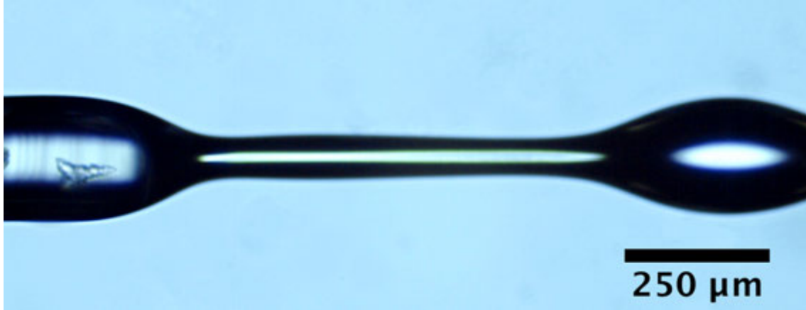
Supplementary Figure 4: Fiber and beads. Solidified jet (fiber) with typical structure shown across all specimens; a central fiber decorated by beads. These beads on a string effect is the consequence of the interplay between capillary, elastic, viscous, and inertial forces 2 . The beads on a string formation dynamics is cutoff by the drying process.
